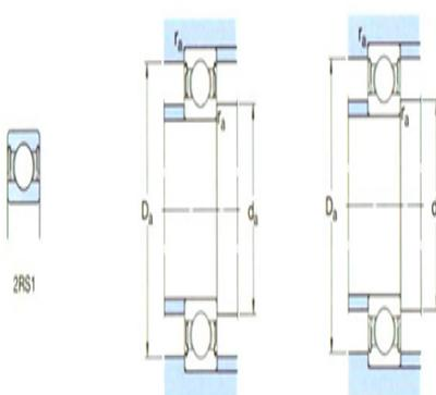
Shoulder gear and chamfer size
