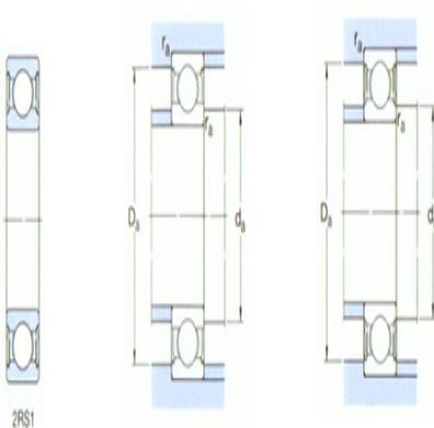
Shoulder gear and chamfer size
