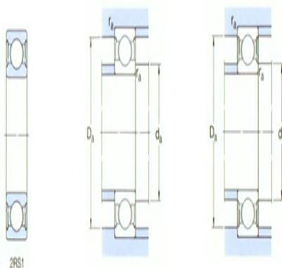
Shoulder gear and chamfer size
