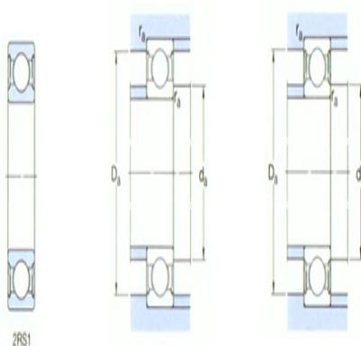
Shoulder gear and chamfer size
