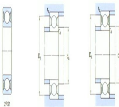
**Shoulder gear and chamfer size mm**
