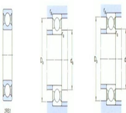
Shoulder gear and chamfer size
