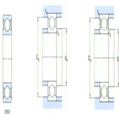
Shoulder gear and chamfer size
