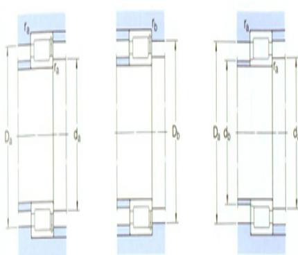
Shoulder gear and chamfer size
