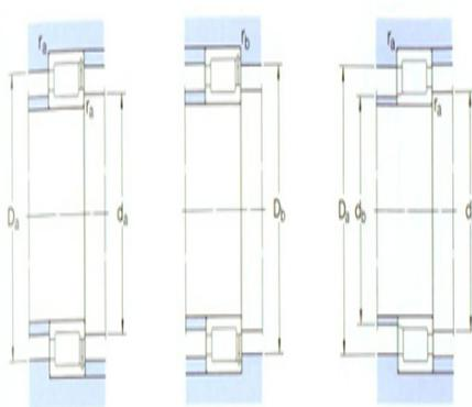
Shoulder gear and chamfer size
