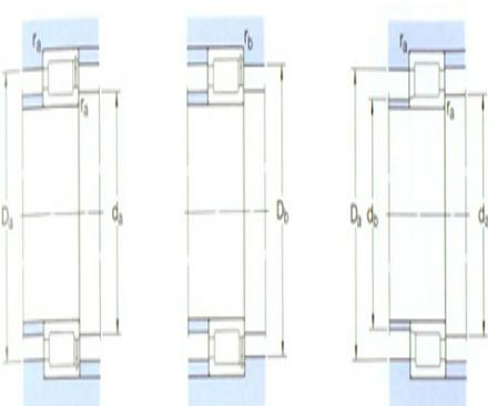
Shoulder gear and chamfer size
