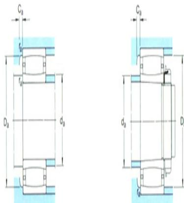
Shoulder gear and chamfer size
