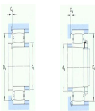
Shoulder gear and chamfer size
