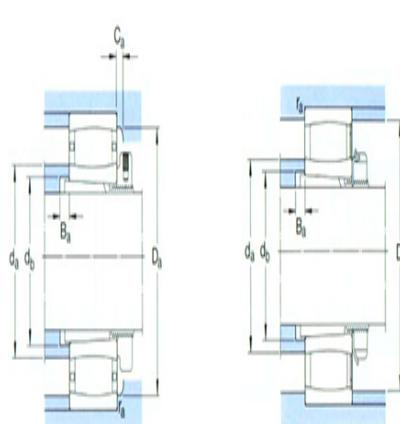
Shoulder gear and chamfer size
